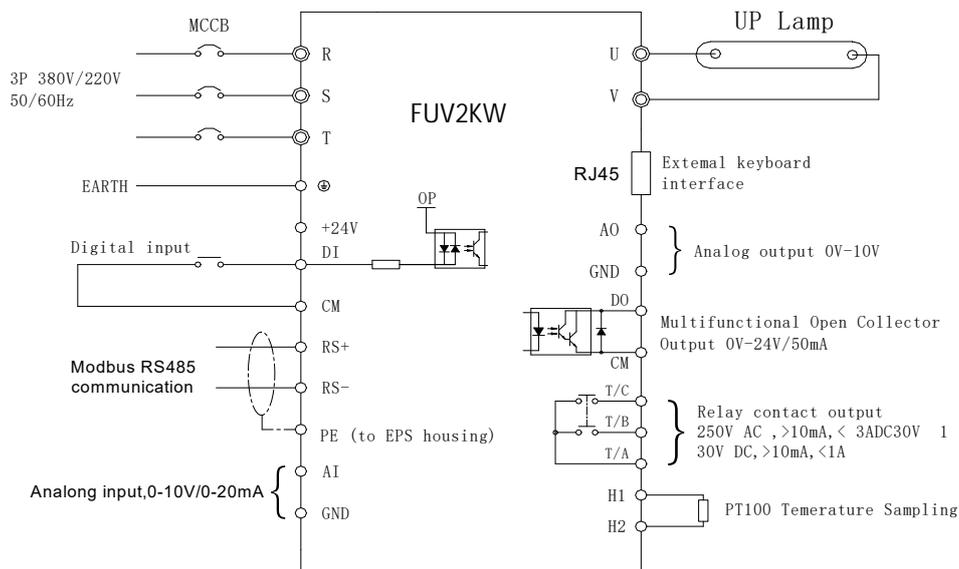
Note: "Ⓧ" Main circuit terminals, "○" Control circuit terminals
